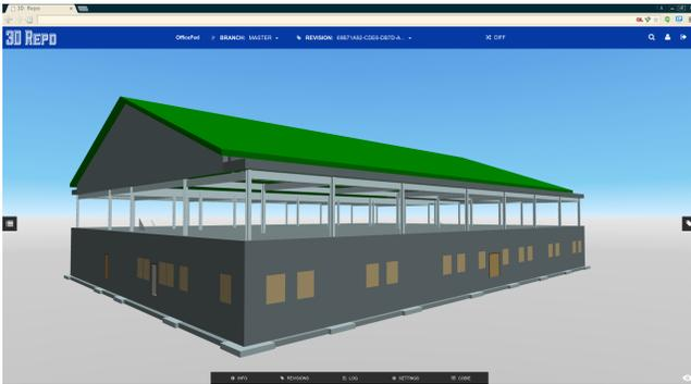
**Figure 6:** Office federated from the Architectural, Structural, and MEP models provided by the buildingSMART alliance initiative. Note that the second storey was hidden to reveal the interior.
