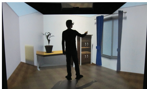
Figure 4: The SweetHome3D output is transferred with our web service to an OpenSG CAVE application which lets the user walk through a 3D representation of the house plan.
