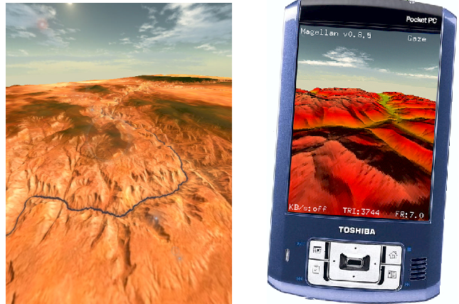
Figure 1: Streaming and adaptive rendering of large terrains. Left: adaptive rendering of the entire Grand Canyon model on a workstation at a target of 25fps, using 440K triangles. Right: adaptive rendering of the Puget Sound terrain model on a PocketPC at a target of 7fps, using 3744 triangles and streamed through an USB2.0 connection.
