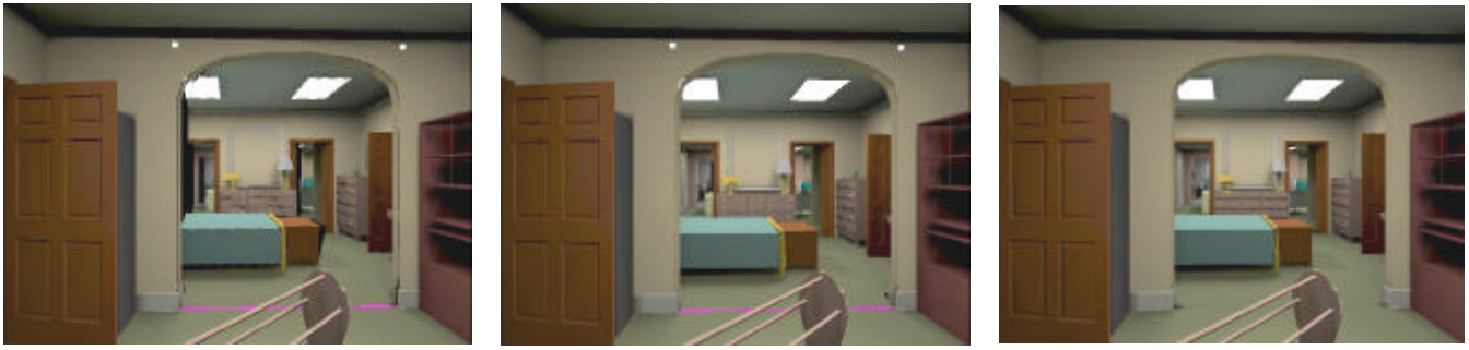
Plate 1. a) Artifacts when only a single image is warped. b) A layered depth image (LDI) does not exhibit the artifacts because it contains surface samples at multiple depths. c) Scene rendered with geometry for comparison.
