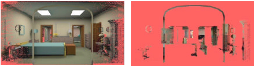
Plate 2. The first two layers of the LDI. Pixels without values are shown in red.
