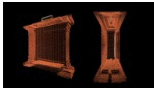
Figure 15. Close-ups of the old clock rendered as point clouds to illustrate back face culling (front and opposite side culled).
