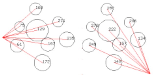
Figure 8. The use of an approximation algorithm to define a priority list. The numbers represent the distances from the desired COP to the center of the spheres. Objects are sorted by decreasing distance.
