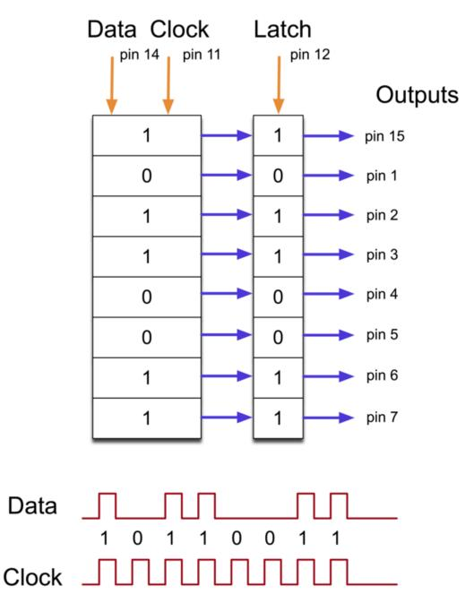
The shift register holds what can be thought of as eight memory locations, each of which can be a 1 or a 0.
