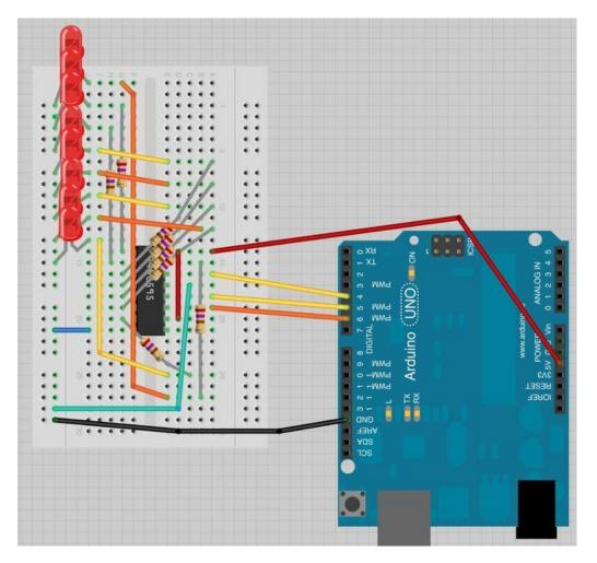
It is probably easiest to put the 74HC595 chip in first, as pretty much everything else connects to it. Put it so that the little U-shaped notch is towards the top of the breadboard. Pin 1 of the chip is to the left of this notch.
