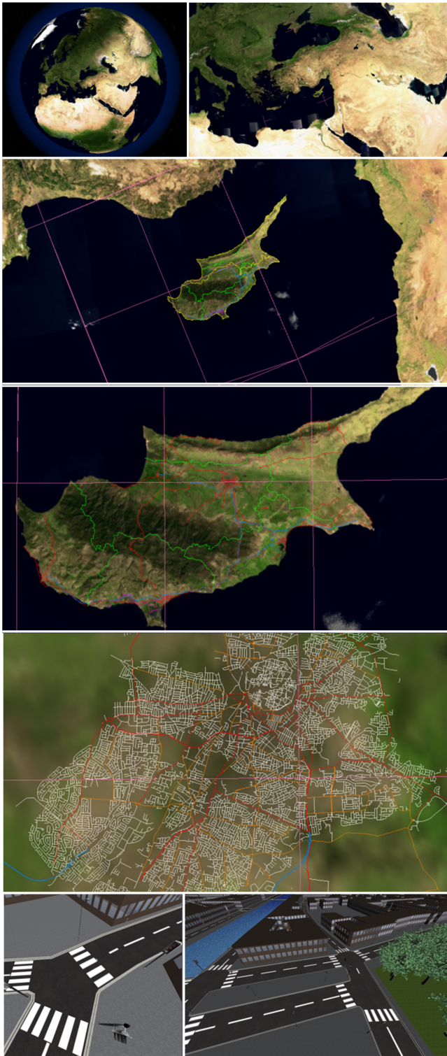
Figure 3: The combination of terrain structuring and visibility optimization with progressive objects and textures allows for a continuous adaptive navigation experience in planet-sized virtual worlds, with visual features ranging from overall country limits to detailed, geolocalized street furniture. In this example data are extracted from OpenStreetMap 3 (127GB database in March 2010) and converted into X3D Earth representation. The buildings are generated using adaptive procedural reconstruction on client-side using the building footprints contained in the OSM database.
