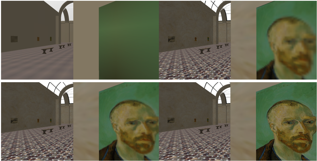
Figure 3. Screen shots from a static viewpoint placed in the museum at different times after the texture downloadings start. Top left: 10s after, at 56Kbits/s. Top right: 35s after, at 56Kbits/s. Bottom left: 1m20s after, at 56Kbits/s. Bottom right: view of highest quality 3s after the texture downloadings start using a local server.
