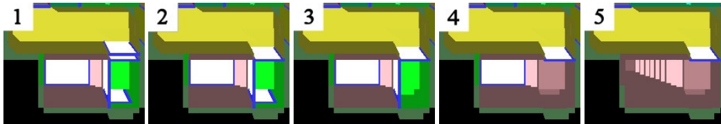
Figure 8: A local view of a CPG during the simplification algorithm. Portals are in white with a blue outline. Our metrics is used to determine which portal should be removed at each iteration. Notice that the last portal corresponds to what we define as a good portal: its neighbouring cell costs are well balanced and it is not in an area easily visible from the scene (it is less visible from the lower floor than the portal at the top of the stairs in picture 3).
