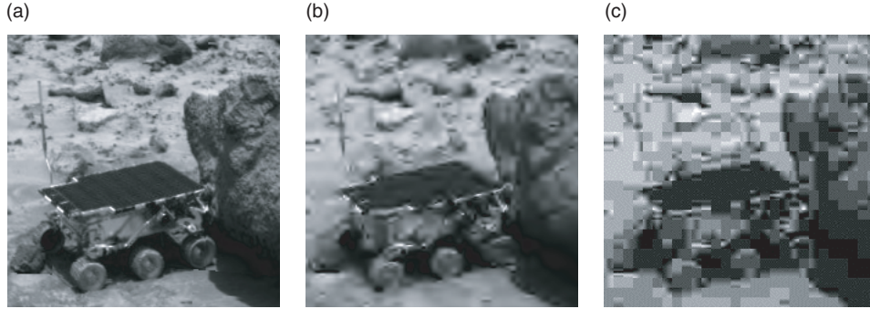
Fig. 2. Details from a larger image: (a) original image, (b) reconstructed image illustrating ringing artifacts after compression to 0.125 bits/pixel using ICER, and (c) reconstructed image illustrating blocking artifacts after compression to 0.178 bits/pixel using JPEG. In this example, the ringing artifacts under ICER are less noticeable than the blocking artifacts under JPEG, even though the image is more highly compressed under ICER.
