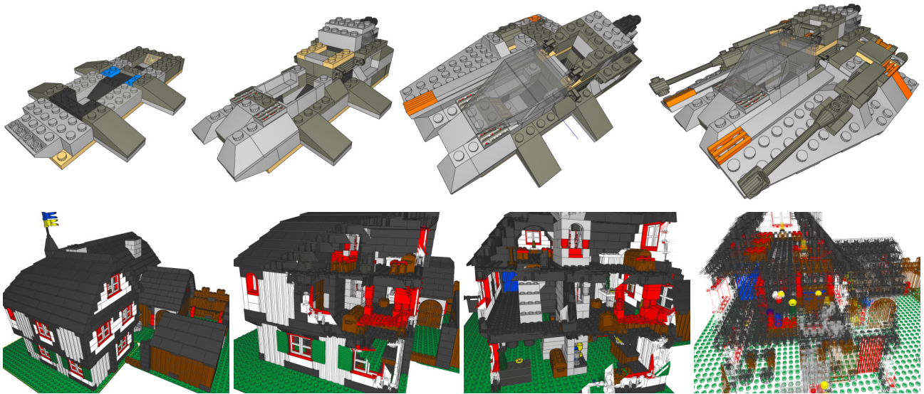
Figure 1.22: Lego models from the LDraw community. The .dat-files can be used as interactive Lego construction manuals as they permit to store stepping information within the model. The highly performant Lego viewer created by Felix Funke (as his Studienarbeit) has a stepping slider. Problematic is the invisible geometry (2d).
