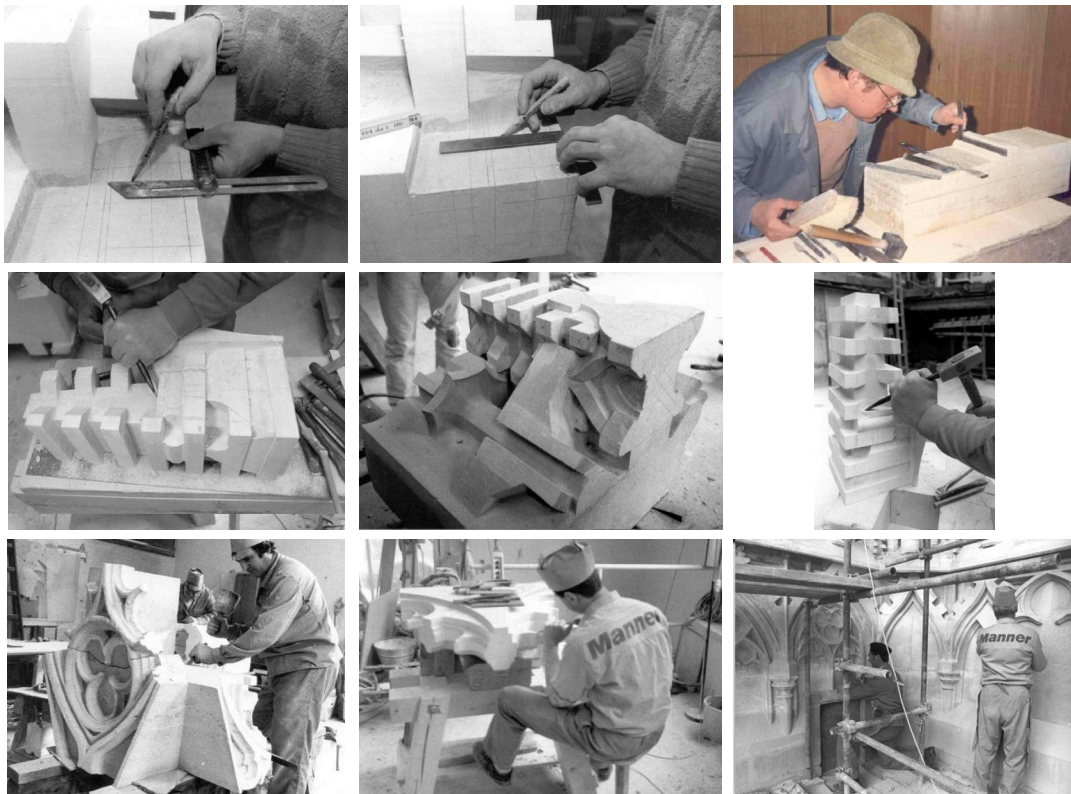
Figure 5.21: For centuries, highly coded construction plans were turned into precise pieces of stone by skilled stone masons. Only through his experience a stone mason can turn a plan like in Fig. 5.19 into a detailed sequence of construction steps. Row 1: The plan is re-constructed in 1:1 scale directly on the stone. Row 2: Plane surfaces and right angles are kept as long as possible, to enable precise measurements. The planes form as tight as possible bounding boxes for the free-form ornaments. Row 3: The final precision is so high that the boundary between different stones is hard to tell. – Images of stone masons at work at the Stephan's cathedral in Vienna, from the Digital European Cathedral Archive at www.deca-forum.net .
