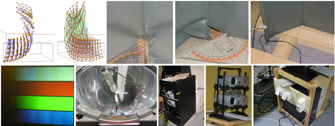
Figure 1.28: Initial problems: The DAVE is a prototype. The magnetic field is ‘dragged’ through the hole in the ceiling (1a,1b). Kai and I take 9 \times 9 \times 6 = 486 measurements in a 25 cm grid for use with the calibration library libTrCalibr2 from Utah. The projection screen starts to tear in the corners and I have to reinforce it (1b-1d). Color bits are spread unevenly over 1st and 2nd turn of the color wheel (2a). Lamps explode until we change to digital image’s open projector case (2b-2d). Torsten adds fast fuses to protect the other projectors when a lamp explodes.
