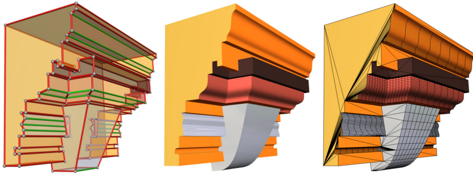
Figure 4.29: Combined B-rep example: Ornamental detail. In classical architecture, most often profiles are rounded only in vertical direction. This can be concisely expressed with combined B-reps by making paths of horizontal edges smooth. The side section, a sharp face, nicely shows the resulting B-spline control polygon.
