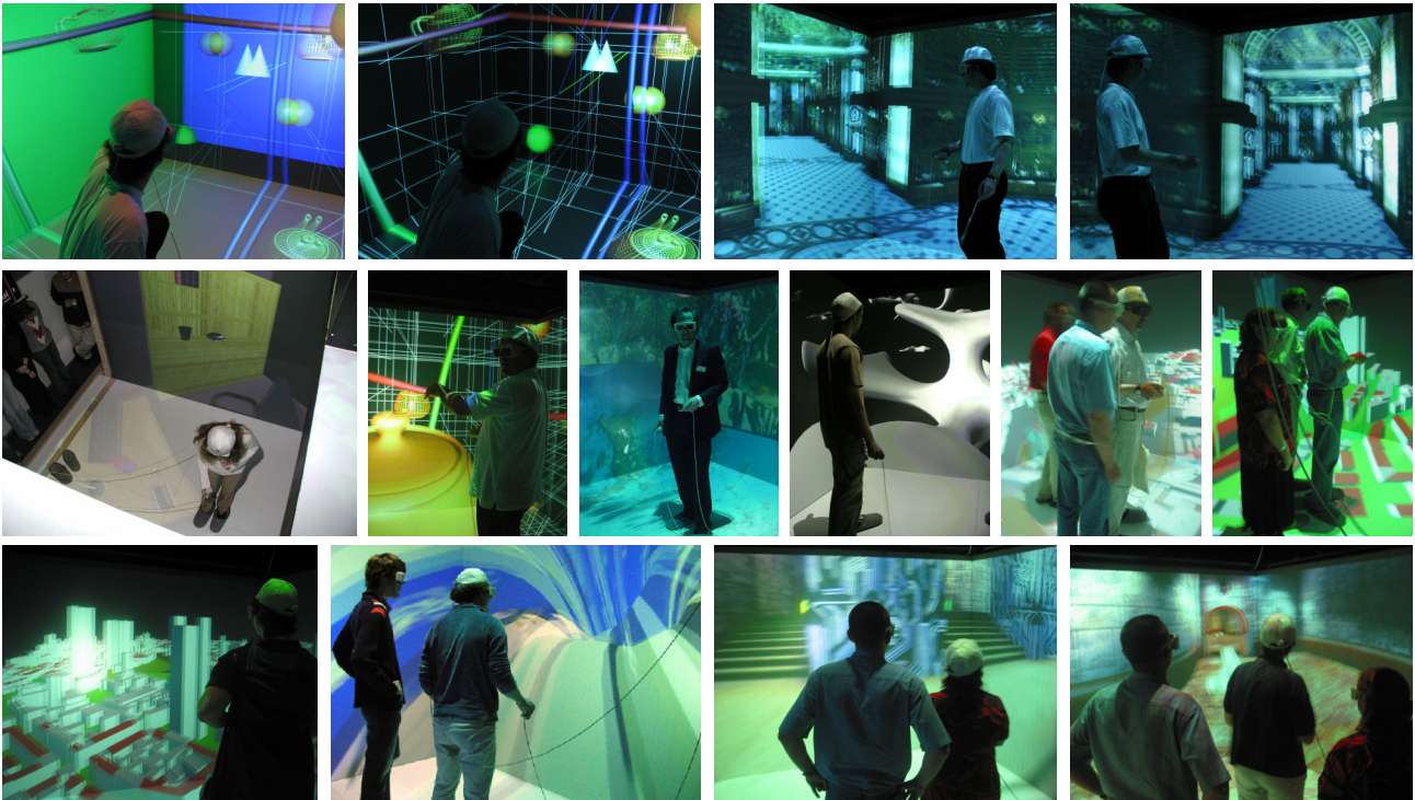
Figure 1.26: Viewer applications in the DAVE. The ‘teapot’ demo (1a-b,2b) is part of the Davelib to demonstrate the easy programming of the DAVE. The fishtank and the Rhino-NURBS-viewer (2c-d) are interactive DAVE applications. Our OpenSG-based VRML viewer (1c-d,2a,2e-f,3a-b) is very impressive with architectural models. It is regularly used for design reviews by architects (3b). Very high quality is possible with specialized walkthrough-software such as Cave Quake III Arena (cq3a) that was ported to the DAVE using the Davelib within a day (3c-d).
