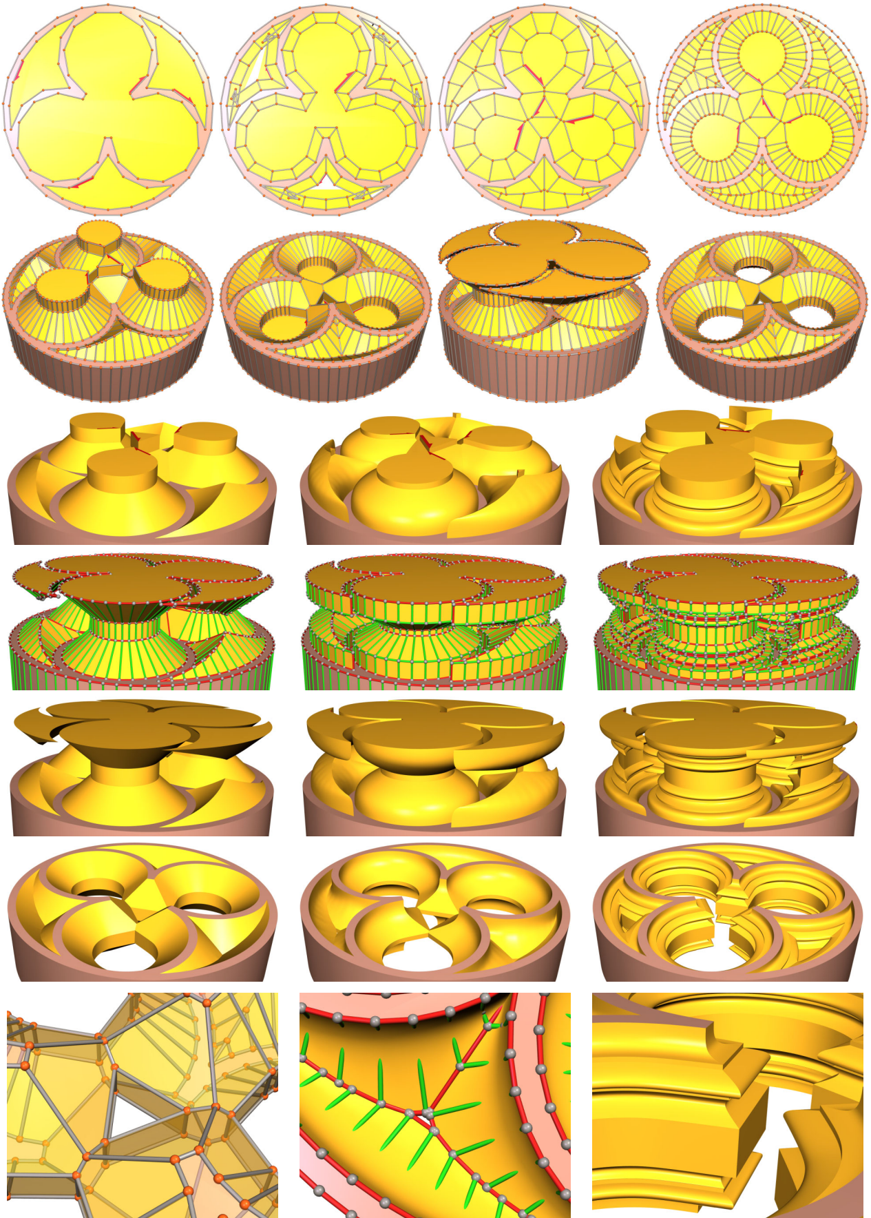
Figure 4.79: Ornamental profile using reversible offset. Highly non-convex shapes require a reversible straight skeleton approach. In the right column (3c-7c) the same profile is used as in Fig. 4.62.
