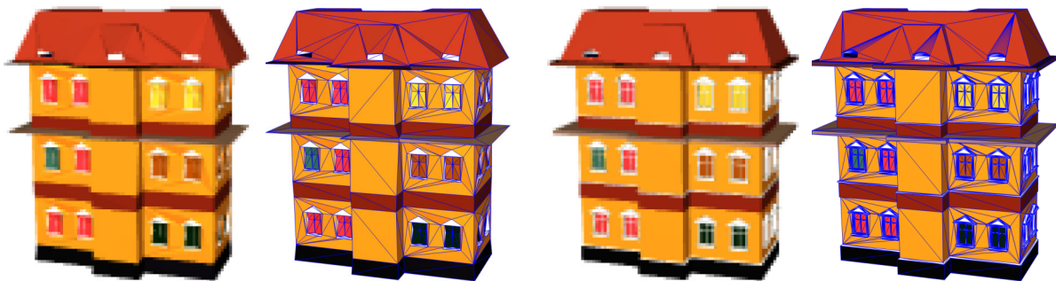
Figure 4.12: Adaptive level of detail with progressive meshes. The low resolution has only 14%, or 558 from 3992 vertices. At a low pixel resolution (a,c), the difference is hardly noticeable, despite the distortion of (b).
