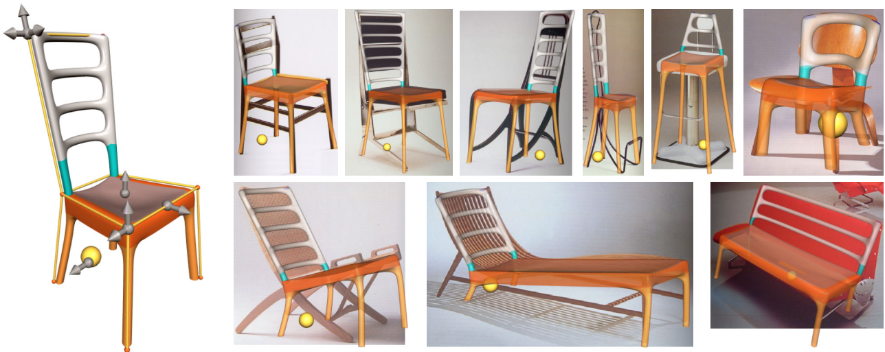
Figure 1.34: Separation of structure from appearance. A generic chair model, parameterized with five 3D points, is adapted to given chairs. The arrows are slider gizmos to move the five control points interactively, so in fact they re-parameterize the DOFs. 12 KB GML code. Note that surprisingly different objects share the same structure.
