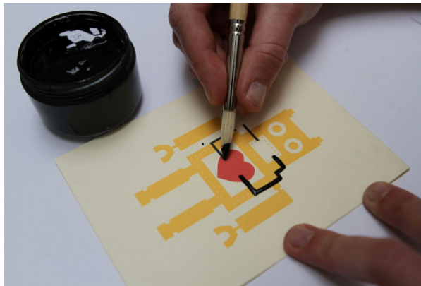
Painting with Bare Conductive Paint and a paintbrush. Image via Instructables.com.
