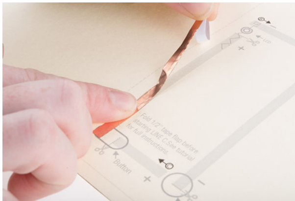
Prototyping with copper tape and a SparkFun template
