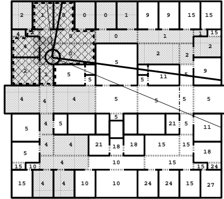
Figure 35: The lookahead cells (stipple gray) contain all objects that can be visible to the observer during the upcoming N frames. Each cell is labeled by the number of frames before it can become visible to the observer.
