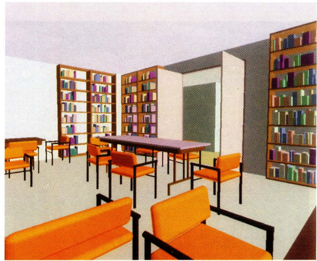
IV. Another typical observer viewpoint. Visible objects are rendered using the highest level of detail for every object (23,468 faces are drawn).
