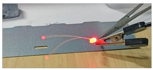
8. The system can be tested by turning the LED on and checking the tiny red lamp that will glow at the tip.
