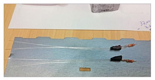
9. The next step is to block the red light that will propagate from the source LED and make the driver's cabin light up red. Use black heat-shrink tubing from electronics suppliers. Choose a size to match the LED and carefully warm it with the soldering iron. It will shrink and wrap around the LED to block the passage of light.
