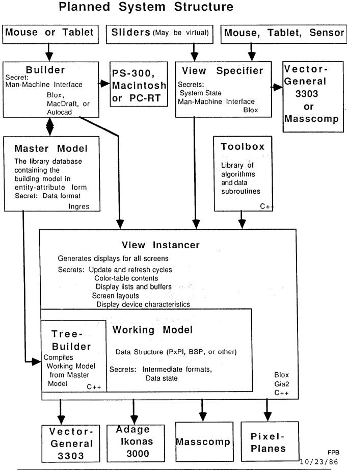
Working Model. The Working Model is now, and will be, entirely encapsulated by the View Instancer, so that new visibility algorithms with their own data structures can be substituted bodily for it without affecting the rest of the system.
