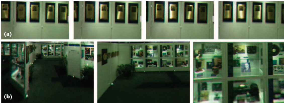
8 Images reconstructed in real time: (a) with specular highlights moving over the surface of the bronze plaques and (b) using prefiltered multiresolution for far-to-near movement of a virtual observer.
